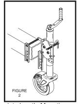
mounting bolts with bolts of appropriate length. Mounting on a round tongue requires modification of the tongue to provide a rectangular area.
