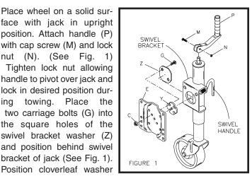
(Y) into the large hole in the swivel bracket with center protrusion of washer facing outward. Position the swivel plate (E) over the end of the swivel handle and the ends of the two carriage bolts. Make certain that the centering protrusion of the cloverleaf washer fits into the center hole of the swivel plate (E). Attach and tighten the two locknuts (C) onto the carriage bolts. NOTE: When swivel handle is disengaged, swivel plate should rotate freely.
