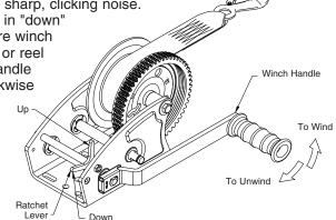
reversing clockwise and counterclockwise. The winch can be converted to wind line on to the underside of the reel. To do this, carefully examine ratchet assembly and remove it from winch. Do not lose small parts. Turn the lever over and reassembly. Do not over tighten bolt. Check operation to insure the ratchet lever rotates fully without binding.
