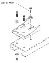
attached using a 3/8" x 3" long bolt and locknut. Use a locknut, not a nut and lock washer. Insert bolt through slots in both reel side plates so that nut is on gear side. Tighten only until snug with bolt in bottom of slot next to reel hub.
