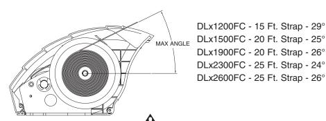
**CAUTION:** Exceeding the maximum strap angle could result in damage to winch cover.
