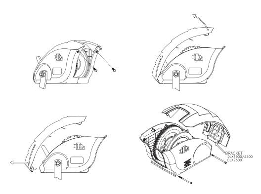
The cover comes off the winch in three pieces. To remove the top cover, loosen and remove the top phillips screws in the front of the cover with a screwdriver. Pull up on the front of the top cover and rotate the top away from the winch. Once the locking tabs are disengaged from the sides, pull the cover straight back to remove.
