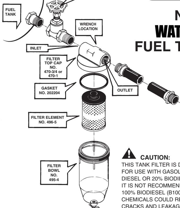
**NOTE:** This filter will not absorb water from fuel containing alcohol.
