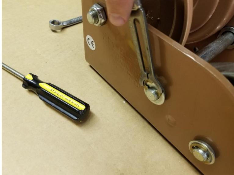
7. Pull the ratchet plunger out into the disengaged position and place the intermediate drive shaft (DD) back into the winch, passing through the Brake Handle Assy (X) and both bearings so that the notch on the end of the shaft is completely visible on the other side of the winch. Place washer (CC) back onto the end of the shaft, and snap on retaining ring (BB) using snap-ring pliers or a retaining ring applicator.
