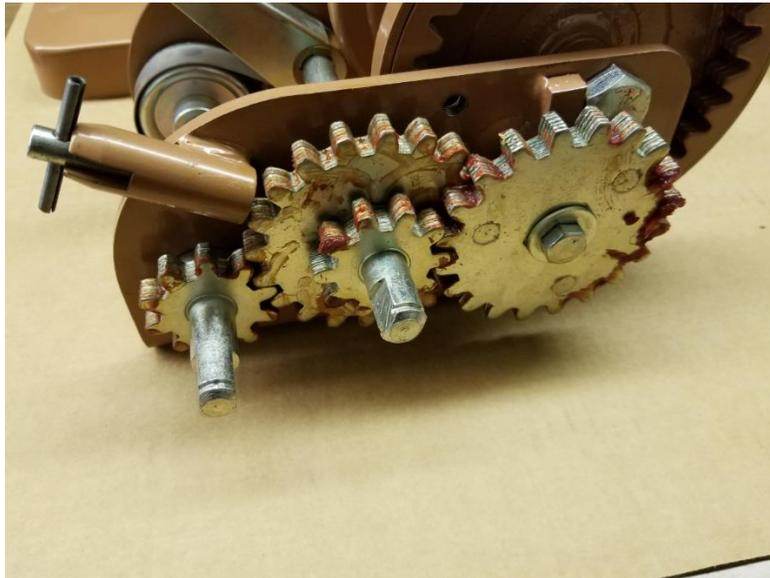
10. The winch should now look like the picture above. The gear cover (C) can now be placed back onto the winch, and can be tightened down by its two screws (S).
